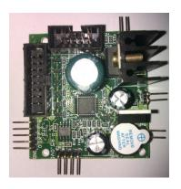
The normal recommendation for the transformer rating for I-SYS weighing scale PCB is 12volts/ 1amps.
