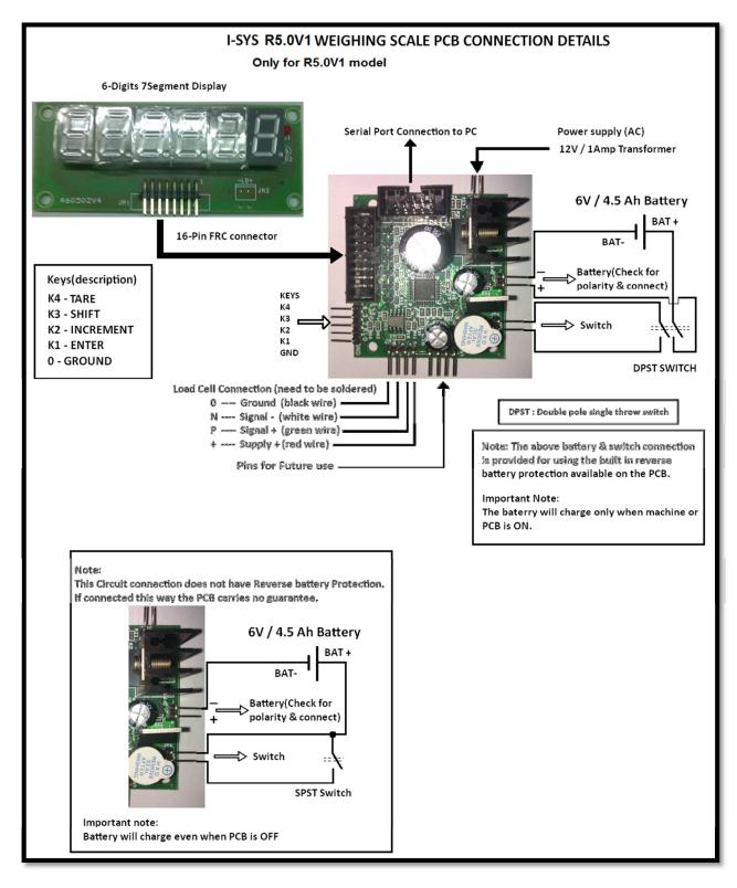
In the unprotected mode you can use a SPST switch. The battery will get charged even when the PCB is in OFF condition. Connecting the battery in the wrong polarity will permanently damage the PCB & the PCB will carry no guarantee.
