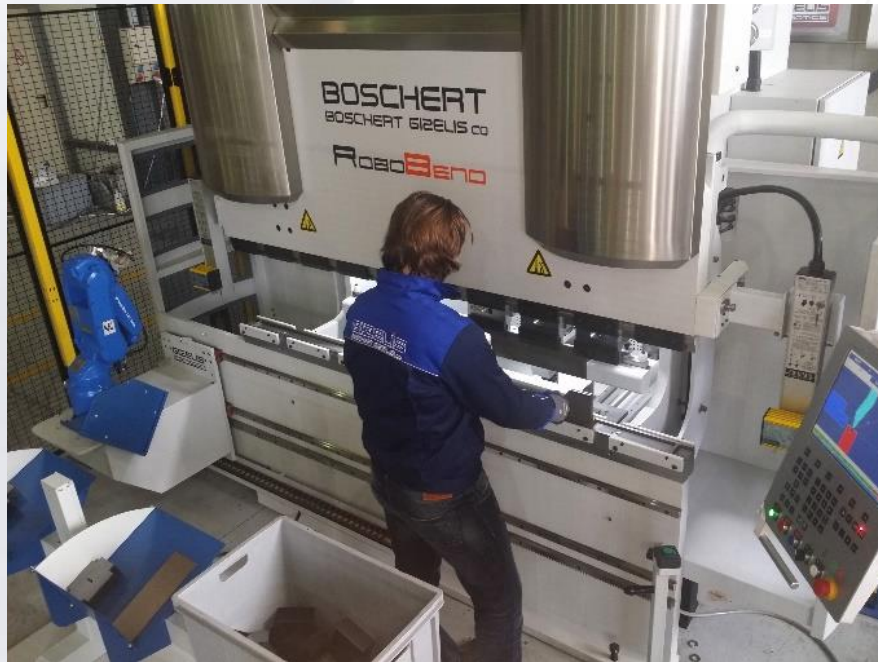
Manual bending possible when robot is on parking position
