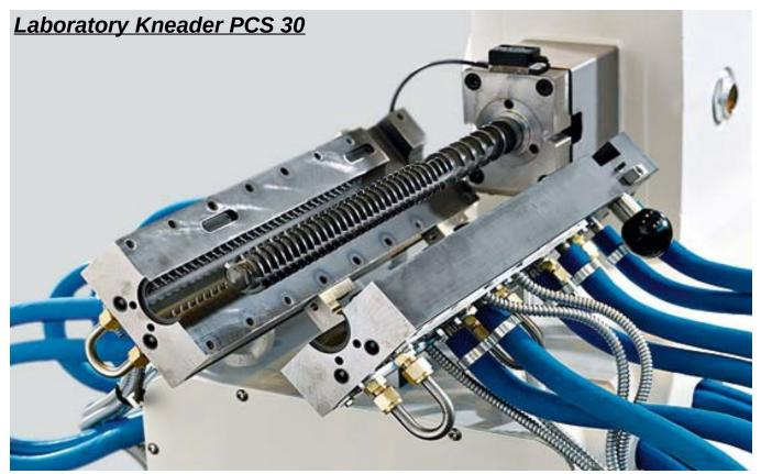
The Clarion make laboratory Kneader PCS 30 is a versatile, compact small scale compounding extruder for research and development, color / shade matching and customer sampling. This easy, economical, user-friendly laboratory kneader offers similar process characteristics as production scale PCS series machines. Samples from 300gms up to 40 kg/h. Based on its process scale-up capabilities it qualifies as a universal laboratory compounder offering a high grade of efficiency and flexibility.
