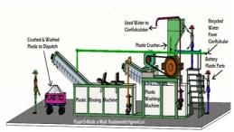
Our Plastic Washing Plant is designed using the cutting edge technology. Capacity of this plant is 150 kg/hour. Plastic Crushing and Washing Plant consists of followings main machines:
