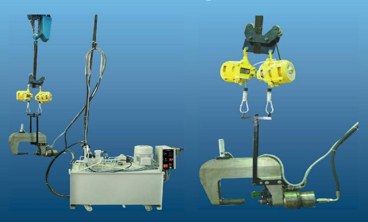
The Portable hydraulic riveting machine is mainly used in all kinds of industry for riveting & pressing etc. Applications - Automobiles & Automobile component manufacturers.
