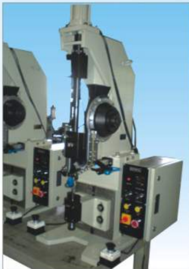
Auto Feed Riveting Machine for Tubular Rivets
