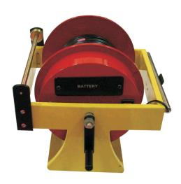
Response is seen on LED plus an audible tone is heard. Features include: Standard cable lengths: 90 mtr. brass electrode is field replaceable. Reel-type spool for lowering cable and electrode assembly. Reel is mounted on a tubular stand. Self-contained 9V battery power supply - no danger of shock from an outside power supply. Battery test. Standard brass electrode. Reel handles are shaped to fit your hands. Accurate to  $\pm 1\%$  of reading. Each
