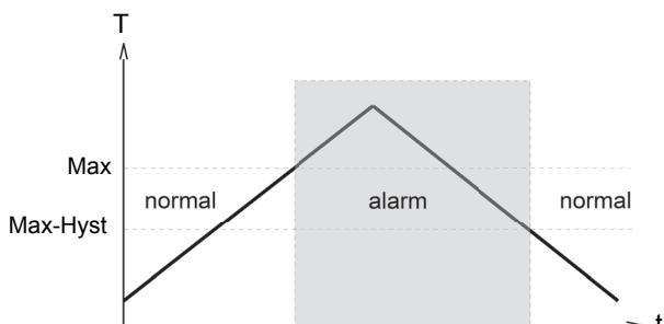
The change to the alarm state is indicated by the integrated red LED and a cleartext in the display. While in the normal state the switching outputs are at the level of the supply voltage; in the alarm state they are at 0 V, so that a wire break would also display as an alarm state at the signal receiver.
