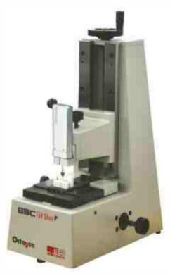
GBC 150 Gold Gauge block comparator with SIOS – laser-interferometric gauging probe of long measuring range 20 mm, resolution 0.001  $\mu$ m and linearity of  $\leq \pm 0.002 \mu$ m at top side and bottom one with the high precision inductive probe
