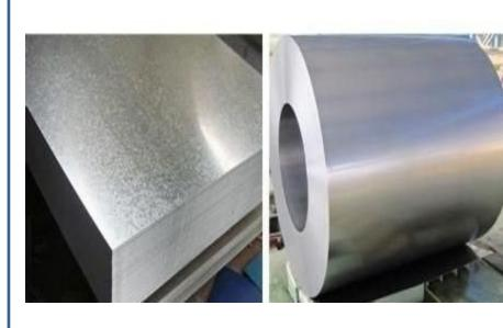
Hot-dip galvanized steel sheets (GI) are Produced by passing the full hard sheet which has undergone the acid washing process and rolling process through the zinc pot, thereby applying zinc film to the surface.
