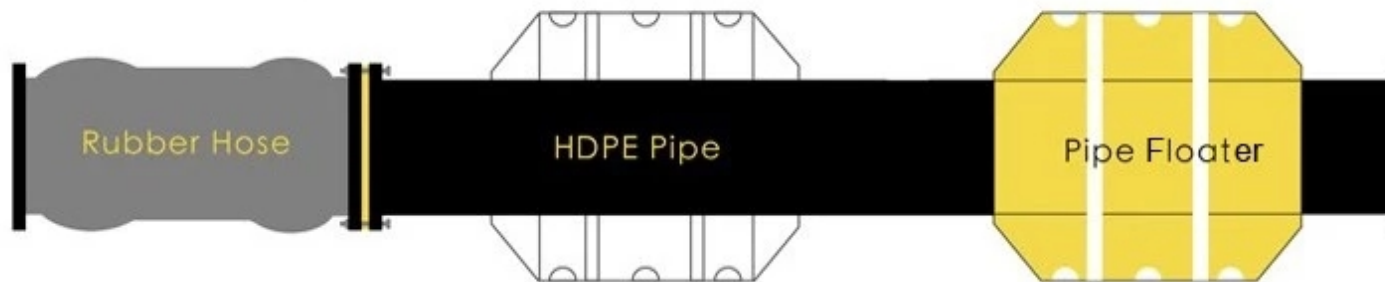
DREDGING PIPELINE FOR CUTTER SUCTION DREDGER
