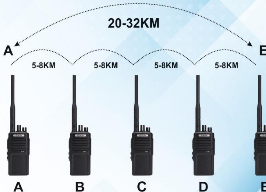
NDMR communication principle
