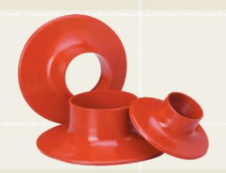
Insulshed is used to increase the surface creepage distance of the cores of cable termination without increasing the tail length. They are also used to avoid continuity during rainy season to avoid short circuiting of the electrical network.
