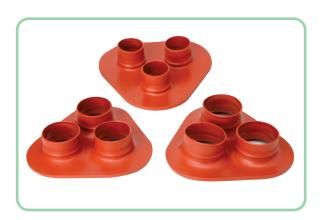
Insulshed is used to increase the surface creepage distance of the cores of cable termination without increasing the tail length. They are also used to avoid continuity during rainy season to avoid short circuiting of the electrical network.
