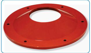
Gala Elastomeric End Seal has been made from specially formulated Rubber Compound and designed to give optimum efficiency to the Curing process by holding pressure to the desired level. It also helps to neutralize the usage of process water/gas by holding the Cable tight during production runs.
