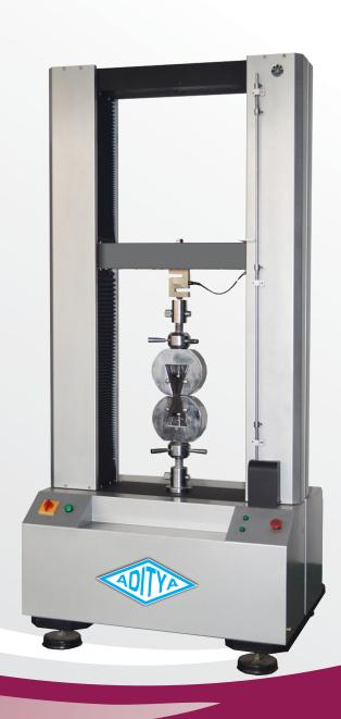
DI make TNE series machines are electronic screw driven machines with precision screw and column construction and variable speed drive. These are high precision, high performance universal testing machines, maximum capacity up to 100 kN. With the help to computer and micro-computer, all the operations from control of load to processing of data are carried out with excellent performance, reliability, flexibility and easy operation.
