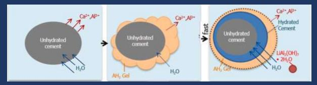
Mycroblock FN accelerators increase the solubility of calcium ions in the mix, promoting faster hydration of cement particles. FNs are made up of a polymer backbone with carboxylate groups that help reduce the viscosity of the concrete mix. FNs work by creating a steric effect. The long, flexible polymer chains attach to the surface of cement particles, preventing them from clumping together. This dispersion leads to improved workability and reduces water demand.
