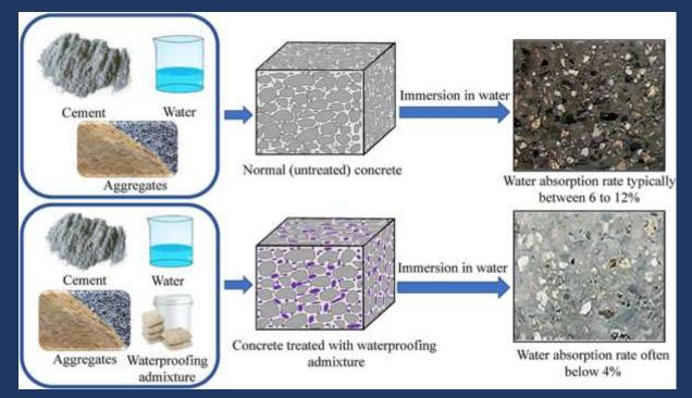
When contact with water, integral waterproofing **Mycroproof AW**+ generates non-soluble crystal throughout the capillaries and pores in the concrete structure creating an impenetrable water barrier to block water passage from positive (exterior) side, negative (interior) side or from within the concrete itself. Mycroproof AW+ also reacts with water to seal cracks that develop in the concrete over time.
