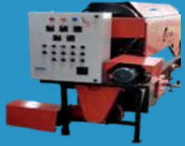
Biomass Torrefaction Plant (Charcoal Plant)
