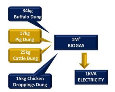
62.5M3 BIOGAS IS REQUIRED PER HOUR TO RUN OUR 62.5KVA BIOGAS GENERATOR SET
