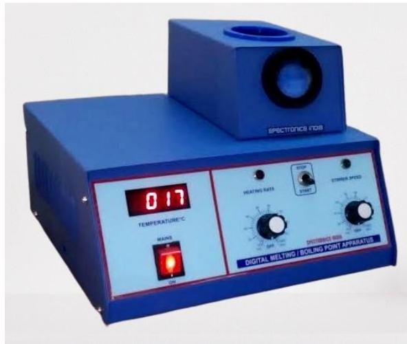
Digital Melting Point Apparatus is a compact instrument designed for accurate determinations of Melting Points of solid samples.
