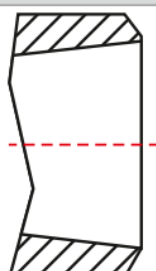
End Prepared for Welding
