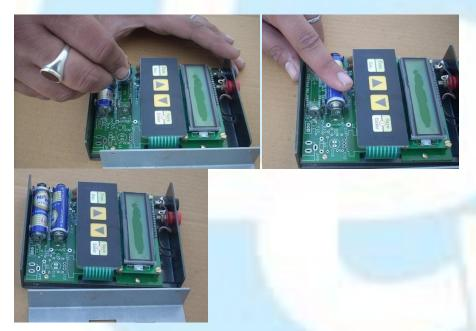
Now place the front panel as was opened & screw back all the four side screws.
