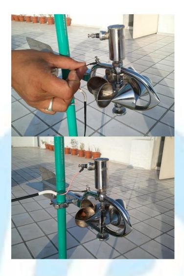
Now connect other of sensor cable to Digital Water Velocity Indicator as shown below
