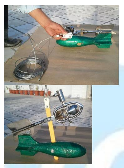
Now fish-weight assembly is ready to lower to the river stream for measurement.
