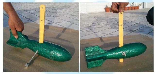
Now insert water current meter to the hanging plate & insert the bolt followed by screwing nut to fix it
