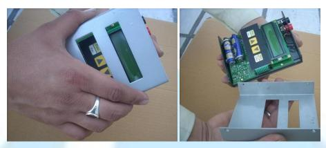
Now remove the old batteries & replace with the new batteries. Make sure while inserting new batteries polarity of battery should be in the same direction as marked on motherboard as shown below.
