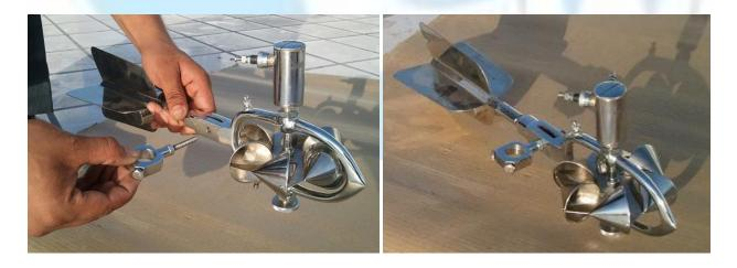
Now Insert the sensor coupler to the wading rod, tighten side bolt to make it gripped perfectly with wading rod as shown below.
