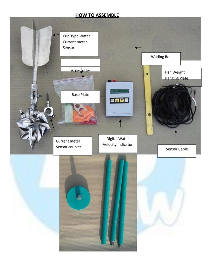
First of all place the wading rod at the center of base plate & insert by screwing the wading rod as shown below. After fixing wading rod (as per the depth requirement) to base plate place it on the floor.
