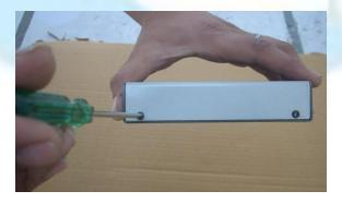
Now open the front panel by pulling the panel in upward direction. Here you will find batteries installed in the instrument motherboard.
