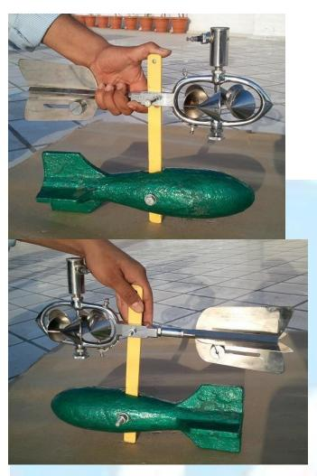
Now attach hanging wire to the fish-weight hanging plate insert the bolt followed by screwing nut to fix it as shown below
