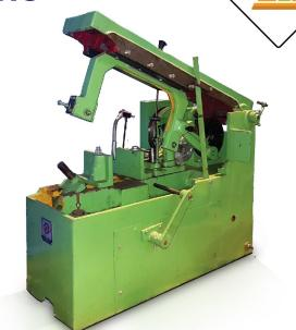
BED: The bed is of rigid casting with wide through for collection of coolant, swarf and also houses the V-Belts drive. Bed is single piece casting.
