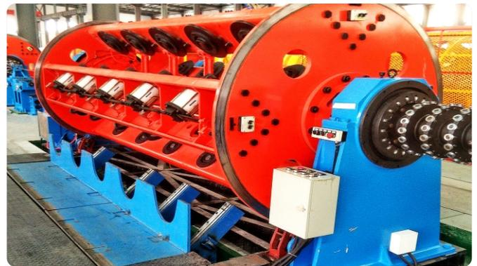
Automatic PLC Controlled Stranding Machines for Conductor making
