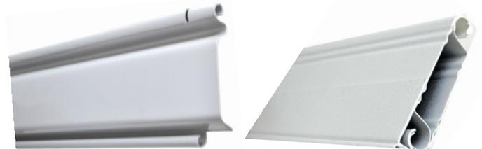
Depending on the size and the application, we use single skin (Left) or double skin (Right) precision cold rolled galvanized steel slats (0.8mm, 1.00mm & 1.2mm thickness). We provide a standard range of powder coated colors.
