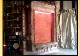
Testing a fire shutter (4 hours) to BS standards for fire rating.
