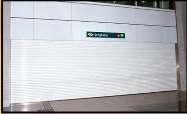
10m wide fire shutter for MRT use, powder coated to client's chosen color;
