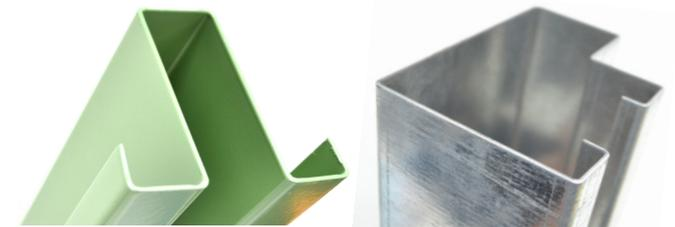
Guide rails for (Left) concealed applications or (Right) exposed wall fixed applications are made from 3mm thickness galvanized steel.
