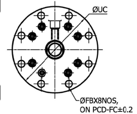
Simran Flotech Millduty Std Front Circular Flange Mtg As Per ISO 6020-1 MF3 Mtg
