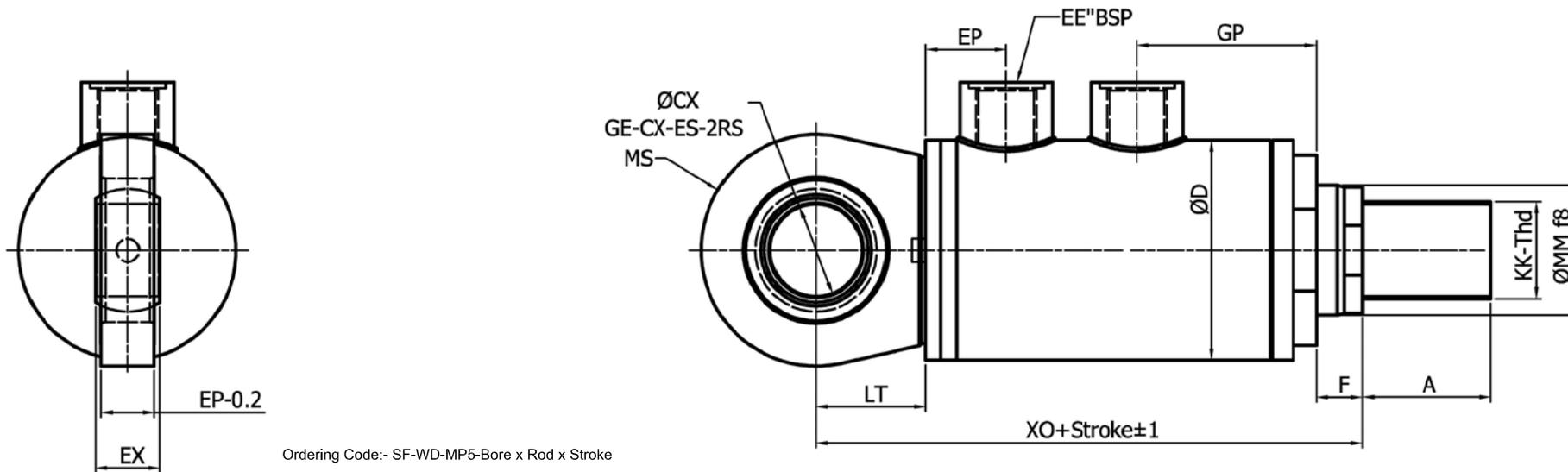
Ordering Code:- SF-WD-MP5-Bore x Rod x Stroke
