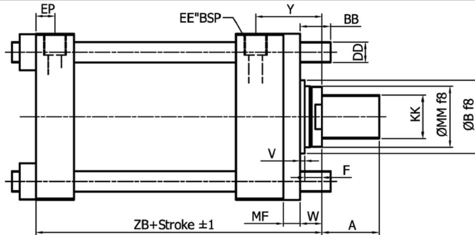
Ordering Code:- SF-TT - MX3 - Bore x Rod x Stroke
