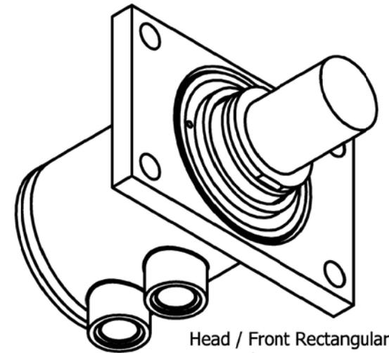
Head / Front Rectangular Flange Mtg. ISO ME5 Mtg.
