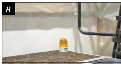
(H) An warning audio alarm and strobe light are added safety features, that activates when the system is being operated.
