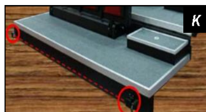
(K) Obstacle sensors mounted on the leading platform automatically stop operation when an obstruction is detected and resumes when clear. Additional safety measures include sirens and warning lights.
