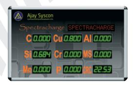
**SPECTRACHARGE** is a magnified display to show the addition of charge on shop floor. **Spectraview** will display the report from the spectrometer readings and **Spectracharge** will display what addition is required if desired value is less or greater than expected.
