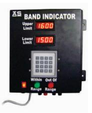
It is a microcontroller based, wall mountable unit which is used for giving audio and visual indication for Within Range Temperature Reading (Green Lamp) and Out of Range Temperature Reading (Red Lamp + Hooter). It has facility to enter Upper Limit Reading and Lower Limit Reading of Temperature.
