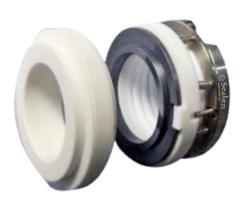
Teflon Bellow Seal TBR 520 Series are designed for extreme corrosive chemical applications including concentrated acids, salts, strong oxidising and reducing agents & chemically active organic compounds. All components which come in contact with the liquid to be sealed are made of chemically inert material. Metallic components, clamping 'ring and springs are located outside the media.
