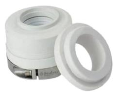
Teflon Bellow Seal TBM 510 Series are designed for extreme corrosive chemical applications including concentrated acids, salts, strong oxidising and reducing agents & chemically active organic compounds. All components which come in contact with the liquid to be sealed are made of chemically inert material. Metallic components, clamping ring and springs are located outside the media.
