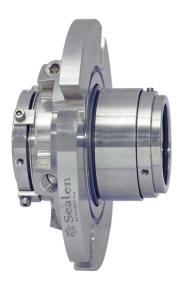
Multi Spring Out Of Product Cartridge Seal MSOP/C 160 Series is a multi spring cartridge construction factory assembled slide on seal specially designed and developed for slurry application. The springs are protected from the media by means of dynamic O ring. This seal requires tightening of stuffing box studs, nuts and detaching of location plate before starting the equipment. No dimensional measurement are to be done at site. Seal can be easily installed by a unskilled person.
