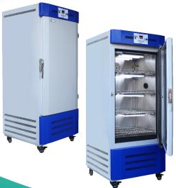
SaiLab Equipment's Plant Growth Chamber is an environmental test chamber that allows plant growth experiments under laboratory conditions. The top-end model has been made sturdy with an all-stainless steel body. It gives Humidity control between 40% and 95% along with temperature control of 10°C to 60°C. The humidity and temperature can be controlled with a micro controller. With the chamber's capacity of up to 1000 litres, the plant growth chamber meets all safety and compliance standards.
