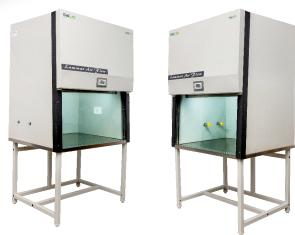
SaiLab Equipment's Laminar Air Flow is designed to prevent the contamination of clinical or laboratory objects from unwanted and foreign particles. The MS Powder-Coated stainless body has a HEPA filter that allows air distribution via straight layers. With sliding doors and transparent glass panels, it makes it easy to view objects. The pre-filter is not washable and must be replaced occasionally. The filter retains particles up to 0.3 microns and runs with low sound.
