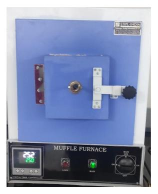
Usage: The **Laboratory Muffle Furnace** units are utilized in general purpose heating in laboratories, ashing tests on wool, rubber, fibers or fabrics, heat treatment requirements for gears and various research facilities in chemistry and physics.
