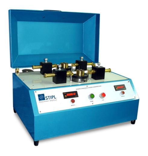
Usage: determines the folding resistance of paper, according to the Louis schopper principle.
