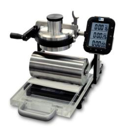
Usage: for measuring water or oil absorption of paper and board.
