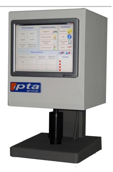
Usage : for measuring the ISO Brightness , colour , colour difference , fluorescence and opacity of paper.
