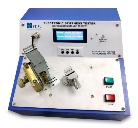
Usage: for measuring the bending resistance of paper, board or plastic.
