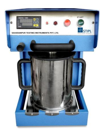
Usage: for disintegration of pulp suspensions according to standardized conditions.
