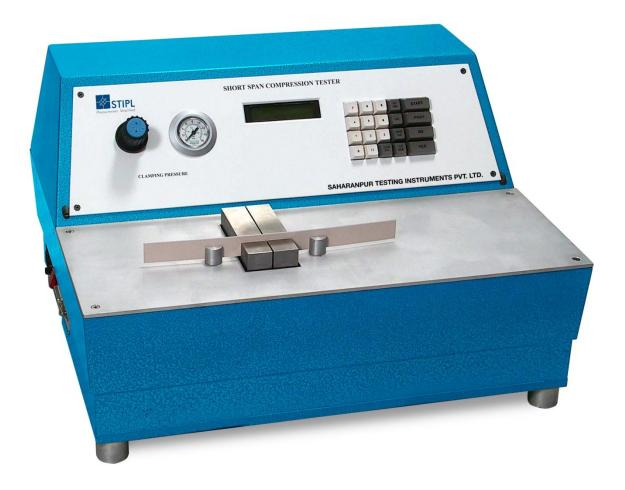
Usage: for determination of compression strength and compression index on paper and board samples .
