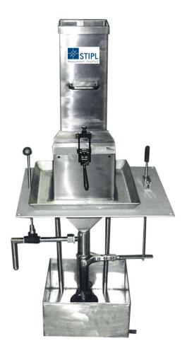
Usage : for the preparation of laboratory sheets of pulp for paper testing .
