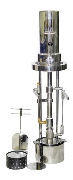
Usage: for the preparation of laboratory sheets of pulp for paper testing.
