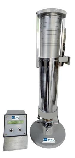
Usage: The Smoothness, Porosity and Softness Tester is intended for testing the average Smoothness, Porosity and Softness of paper and films
