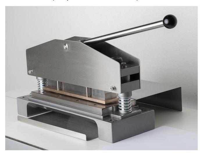
Usage: For preparation of test pieces towards use in tensile strength tests size 15mm x 300mm.
