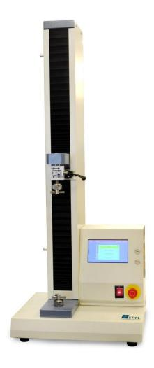
Usage: For the determination of tensile resistance of paper in dry state, elongation and tensile energy absorption in paper or tissue.
