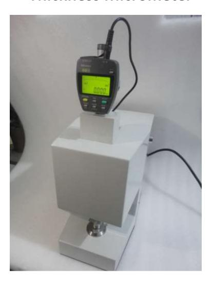
Usage: for measuring the thickness of paper and board.
