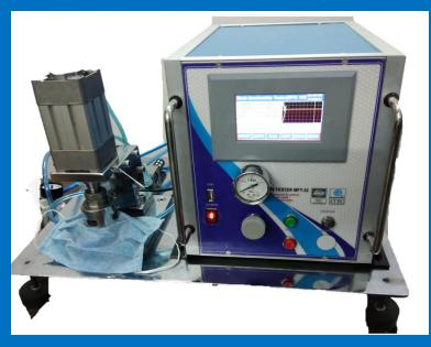
The "PRC" Breathability Tester is based on the principle of differential pressure. It is used to determine the face mask's resistance to airflow. In breathability test, A controlled flow of air is given through the mask, and the pressure is measured before and after the test.
