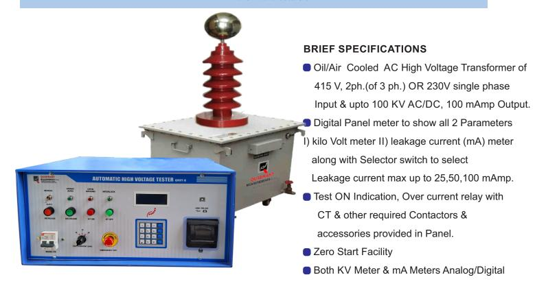
"QUADRANT" make 'Automatic AC/DC HIGH VOLTAGE TEST SET' are ideal to test dielectric strength of
